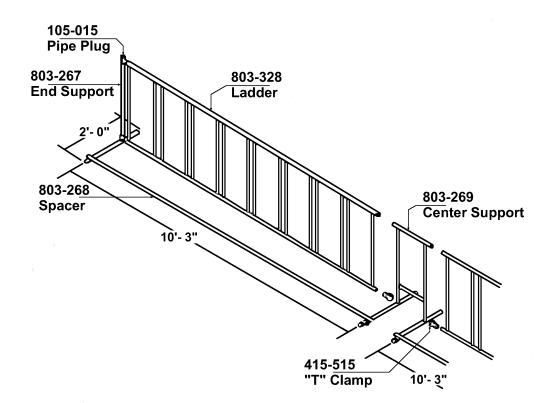
Main Frame, legs and spacers are 1 5/8" O.D. hot galvanized welded pipe with 3/4" O.D. hot galvanized ladder rungs. Spacing between tire posts is 3" center-to-center for small gap,  $8\frac{1}{2}"$  center-to-center for large gap.
